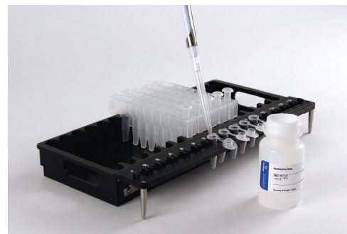
Figure 1. Setup and configuration of deck trays. Nuclease-Free Water is added to the elution tubes as shown. Plungers are in well #8 of the cartridge.
