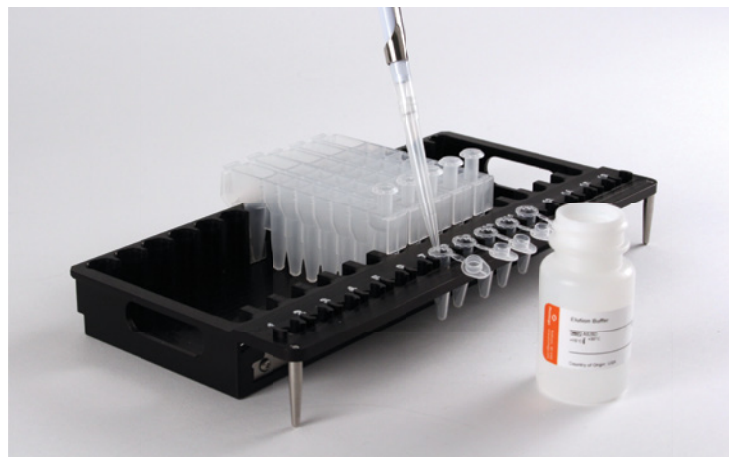
Figure 1. Setup and configuration of the deck tray. The CSC/RSC plunger is placed in well #8 of the cartridge (the well closest to the Elution Tube), and lysates and Lysis Buffer are placed into well #1 of the cartridge.
