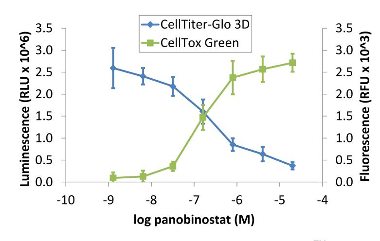
HCT116 cells (RPMI +10% FBS) were seeded in InSphero's GravityPLUS<sup>TM</sup> 96-well hanging-drop platform and grown for 4 days to form ~350 μm spheroids. Microtissues were treated with panobinostat for 48 hours in the presence of 1x CellTox<sup>TM</sup> Green. After recording fluorescence, the microtissues were assayed by adding an equal volume of CellTiter-Glo<sup>®</sup> 3D, shaking for 5 minutes, and recording luminescence after 30 minutes.
