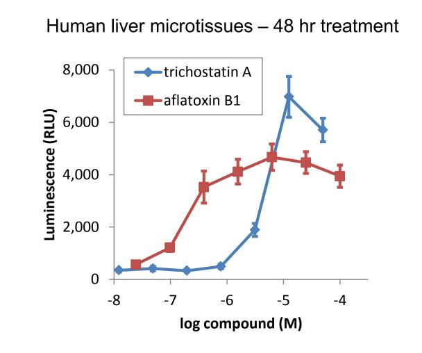
HCT116 cells (RPMI +10% FBS) were seeded in InSphero's GravityPLUS<sup>TM</sup> 96-well hanging-drop platform and grown for 4 days to form ~340 μm spheroids. Human liver microtissues (~275 μm) were provided by InSphero. After treatment, all microtissues were assayed by adding an equal volume of Caspase-Glo<sup>®</sup> 3/7 and recording luminescence after 30 minutes of shaking.
