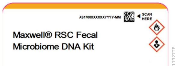
Figure 3. Kit label indicating the method bar code. Scan the bar code shown in the upper right of this label, to start a purification run.
